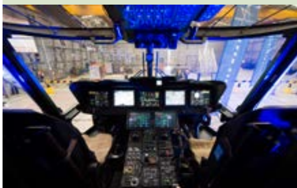
Flight deck of the new Merlin Mk 2 helicopter with touch screen displays
