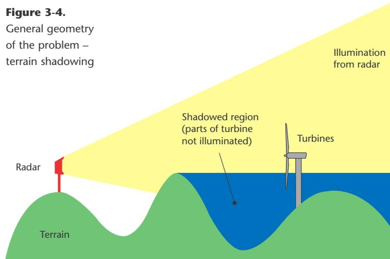
**Figure 3-4.** General geometry of the problem – terrain shadowing
