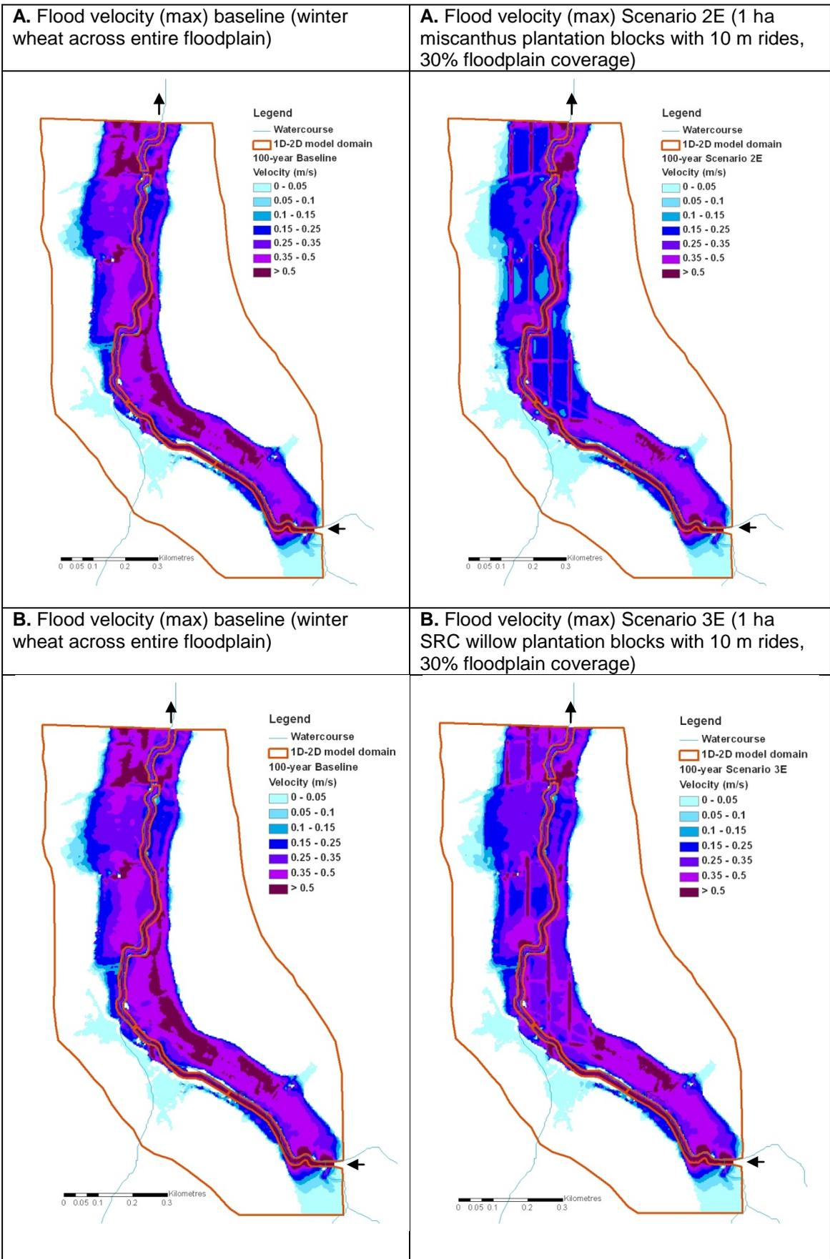
Figure 4.2 River Isle at Ashford Mill – flood velocity patterns
