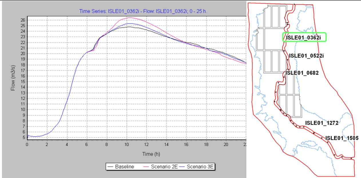
**Figure 4.3 River Isle at Ashford Mill – main channel flood hydrographs <sup>1</sup>**
