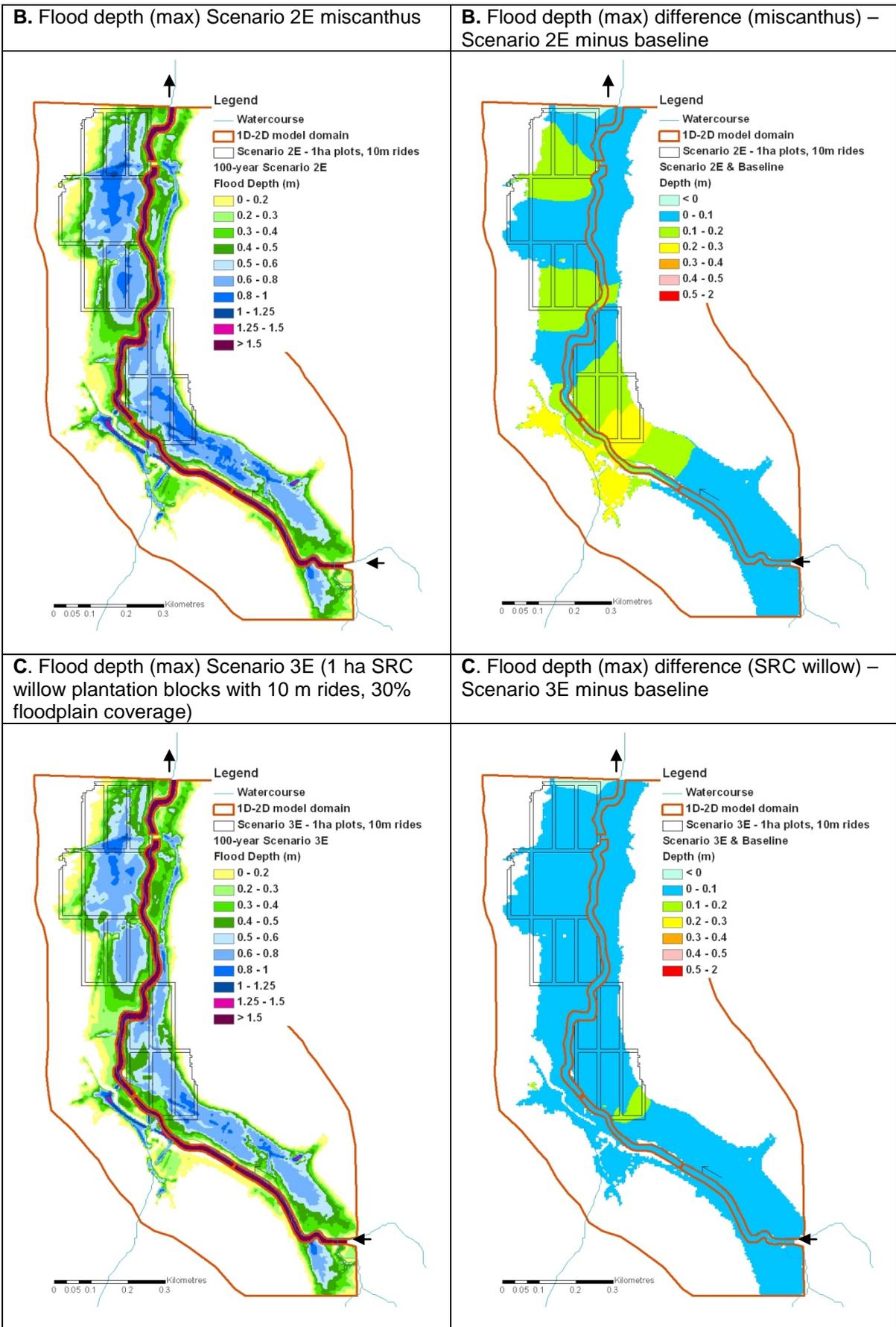
**Figure 4.1 River Isle at Ashford Mill – flood depth patterns**
