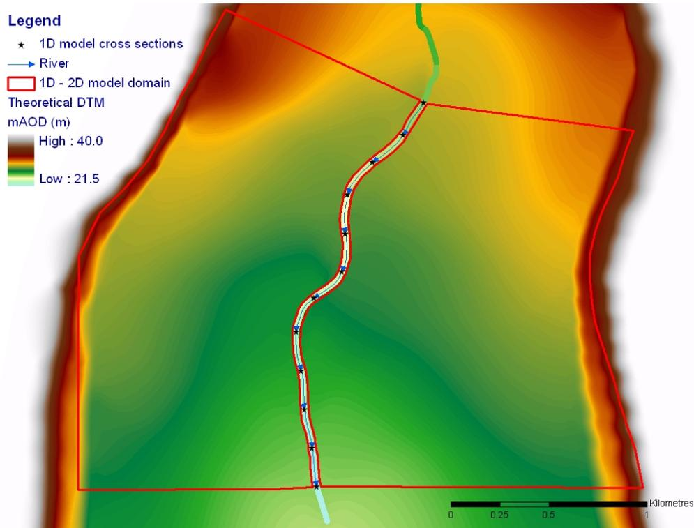
**Figure 3.7 Theoretical model – model layout and topography**
