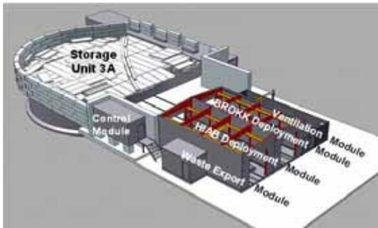
Temporary Process and Contamination Control Modules to be used during installation of biological shielding over the SNF storage tank DSU 3A at Andreeva Bay, NW Russia.
