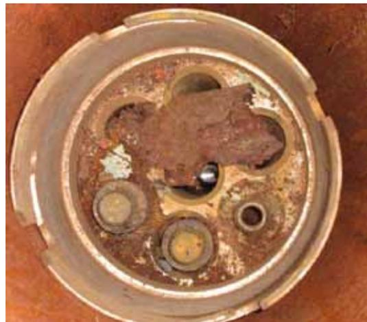
Andreeva Bay – an SNF canister inside DSU 2A. This shows the advanced state of corrosion, debris over the spent fuel assemblies and no shielded canister lid.
