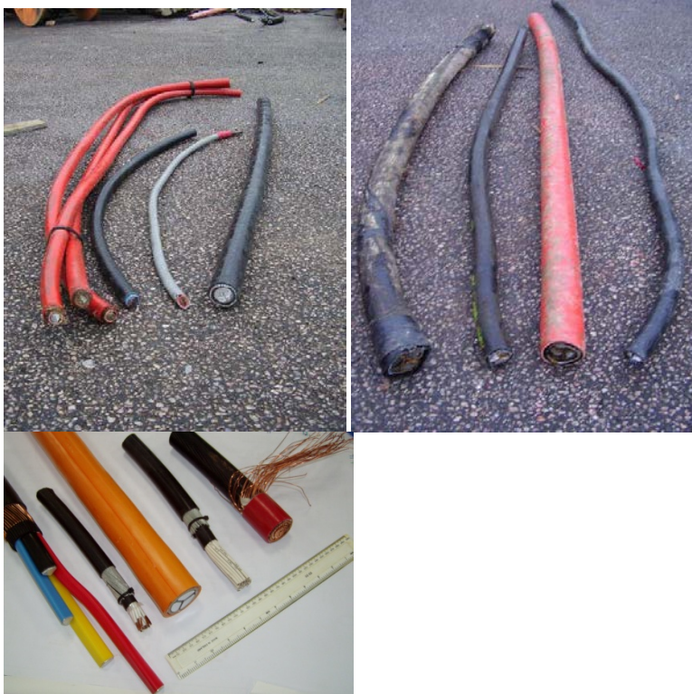
Photograph 5 - Typical underground cable types
