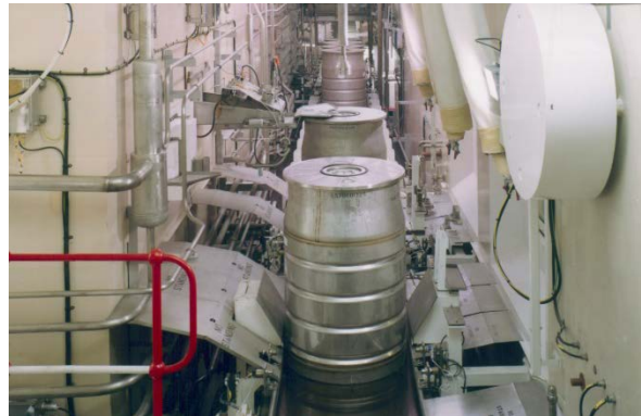
Encapsulation line at Sellafield Waste Packaging and Encapsulation Plant (WPEP)
