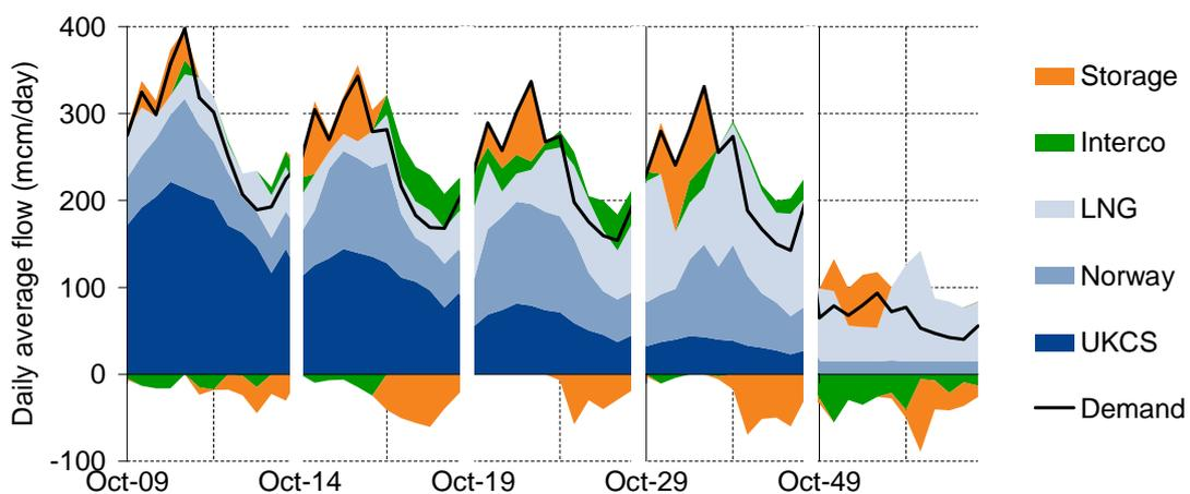
Figure 32 – BAU stress test – LNG flows to GB
