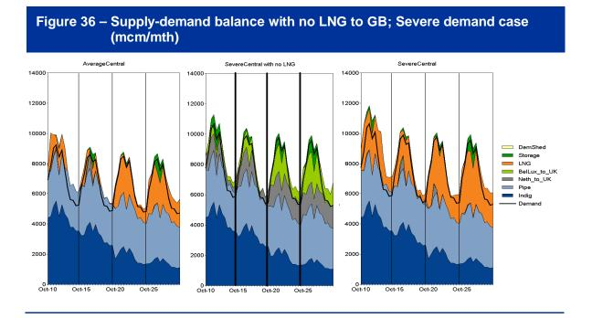
Under the Severe Central case with no supply disruption (right hand chart) there is a small amount of excess supply to demand, which is being exported to the all-island of Ireland and to continental Europe through the interconnectors. There is some usage of storage, particularly in 2025, reflecting the assumption of no additional facilities being built during this period.
