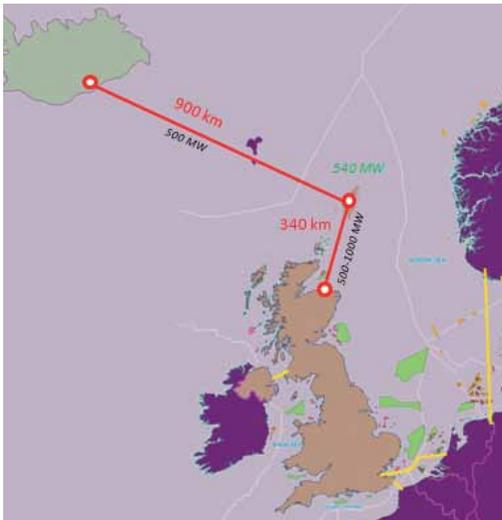
The results of the CBA analysis suggest that, when the electrical interconnection costs are added to the generation capex costs, Icelandic geothermal directly connected to the UK is a potentially cost effective renewable option. The particularly attractive option is the 1,200 km link to Northern Scotland.
