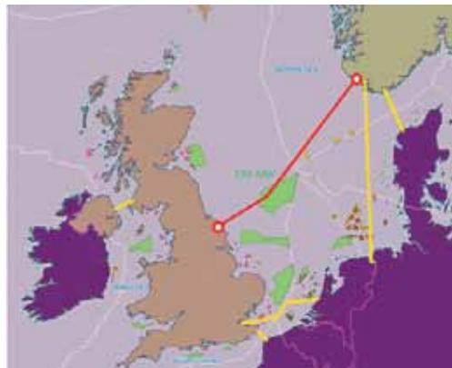
Two cases were analysed in detail to examine the potential benefits of interconnection; a 1000 MW direct interconnection with Norway and the interconnection via Dogger Bank – a 500 MW link from Norway to a 500 MW wind farm at Dogger Bank linked by a 1000 MW
