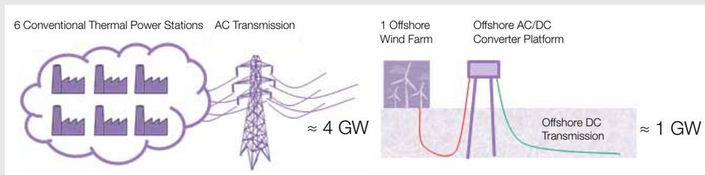
So we conclude that the offshore power hub concept is questionable with current VSC DC technology as one HVDC link per large wind farm is required and so there are no apparent "power hubbing" economies of scale. In addition such aggregation would be limited by system operation safety reasons due to the potential simultaneous loss of generation in case of faults
