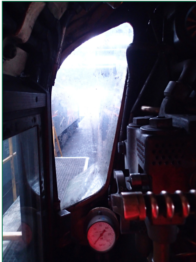
Figure 4: The driver's windscreen on Tangmere – note this image was taken after the incident with the train at a stand and does not show the extent of driver's visibility on 7 March 2015
