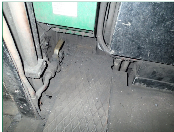
Figure 3: The AWS isolating cock
