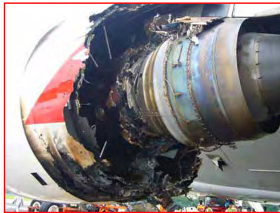
Figure 5: Trent 900 – Uncontained Turbine Disc
