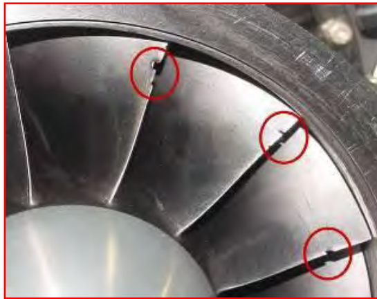
Figure 8: Compressor damage due to FOD.
