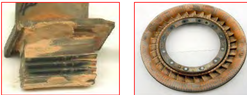
Figure 9: Presence of sand on components post operations in Afghanistan.
