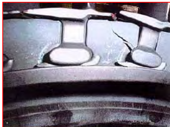
Figure 7: Pegasus Fan Rotor Fatigue Cracking.
