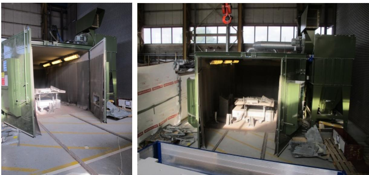
*New blast room installed at BAE's site in Barrow-in-Furness. The facility was built and installed by Hodge-Clemco at a total cost of over £100,000. The reduction in cost associated with purchasing and building temporary enclosures means that the facility will have paid for itself within four years.*
