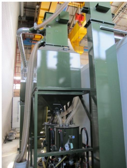
*Extraction (left) and recovery (right) systems installed on the new blast facility. The combination of efficient extraction and air-wash ensure that the blast media is maintained at optimum conditions at all times. This ensures a high quality blast finish (SA 2.5 – SA 3) with minimal clean down time.*
