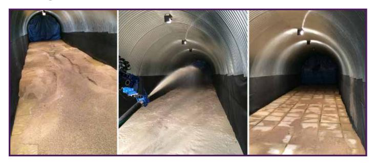
A remotely operated water cannon will wash out sludge from a tunnel section of Dounreay's shaft and silo complex, following a series of trials to test the novel approach.
