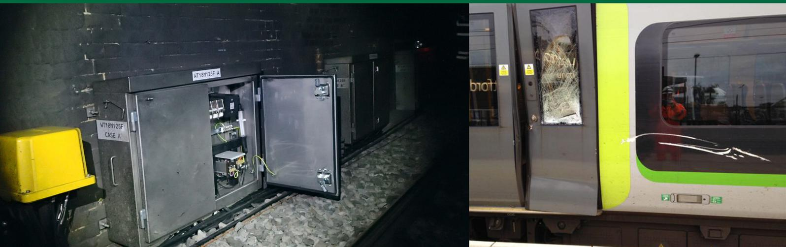
**Train struck and damaged by equipment cabinet door in Watford Tunnel
