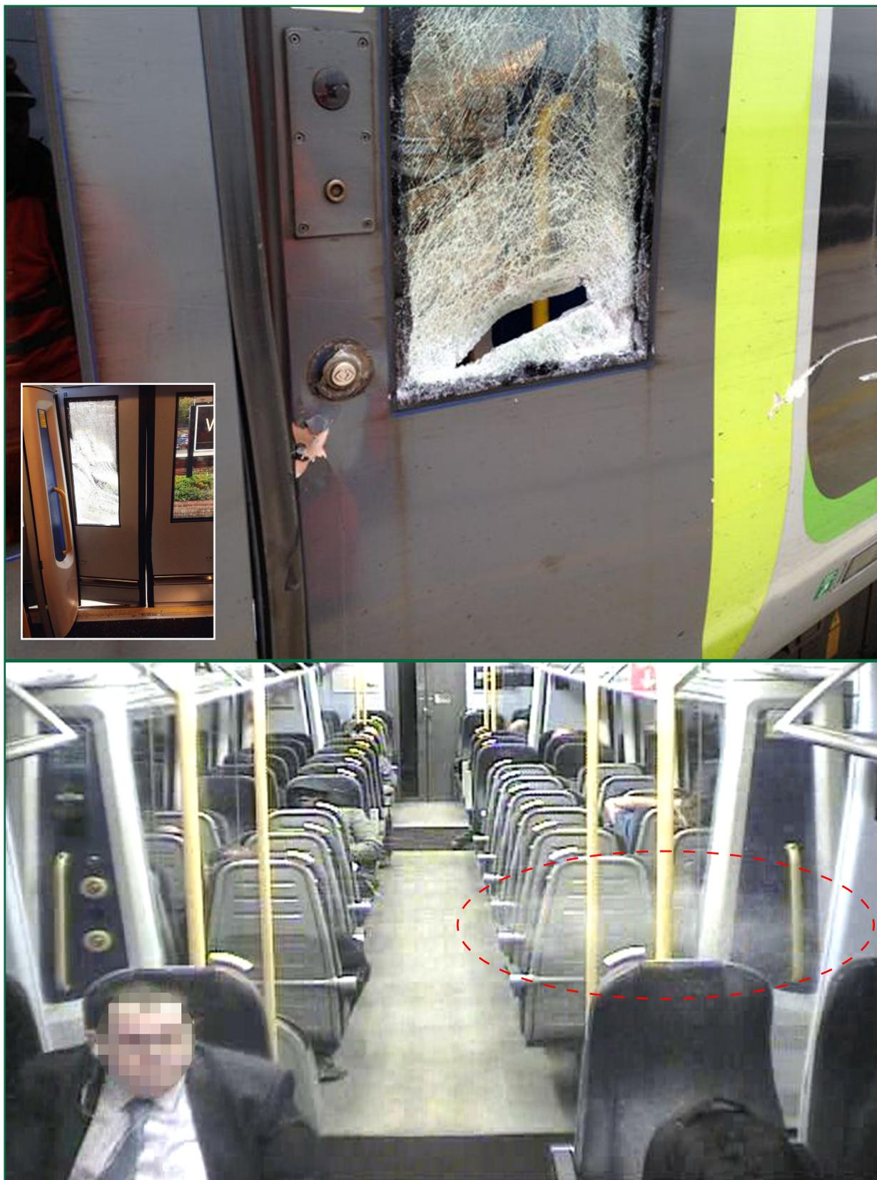
Figures 10 and 11: The damage to the door of carriage 4 and internal CCTV images of the glass entering the passenger compartment
