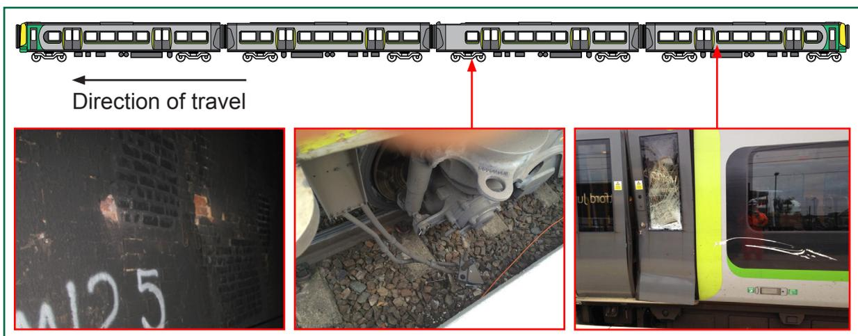
Figures 7 to 9: (left to right) The initial impact damage on the tunnel wall, the equipment on the leading bogie of carriage 3 and damage to the door and body side of carriage 4
