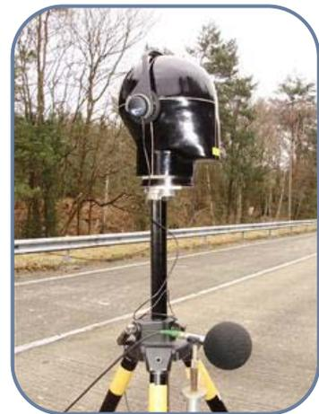
**Figure 3.1: Set-up for binaural audio recording**
