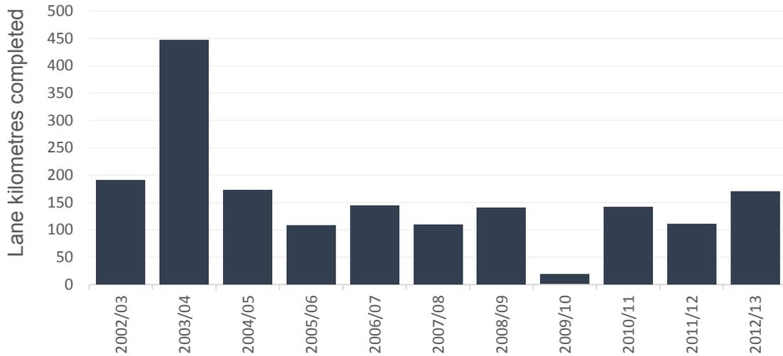
The lane kilometre figures from 2010/11 onward include schemes to introduce different designs of actively controlled motorways known as 'smart motorways'. These motorways use technology to convert the hard shoulder into a running lane, thus increasing capacity.
