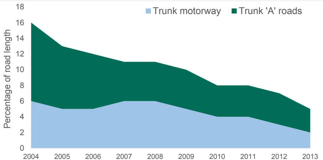
Skidding resistance: Percentage of trunk motorway and trunk 'A' road requiring further investigation <sup>(13)</sup>
