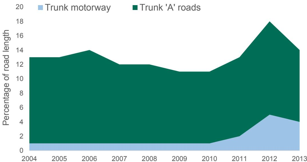
Skidding resistance is a measure of the road surface contribution to the frictional forces developed between a vehicle's tyres and the road when accelerating, braking or cornering.
