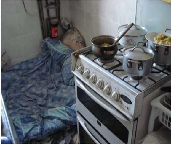
**Note:** bedding adjacent to the cooker adds to the risks of a fire starting and spreading quickly. The lack of adequate workspace also increases the risk of burns and scalds
