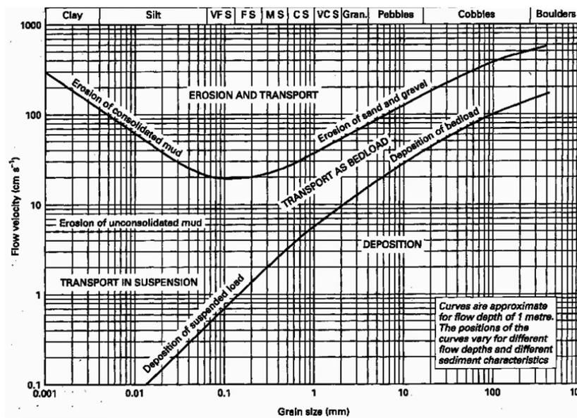
**Figure 5.8 Hjulstrom Curve**
