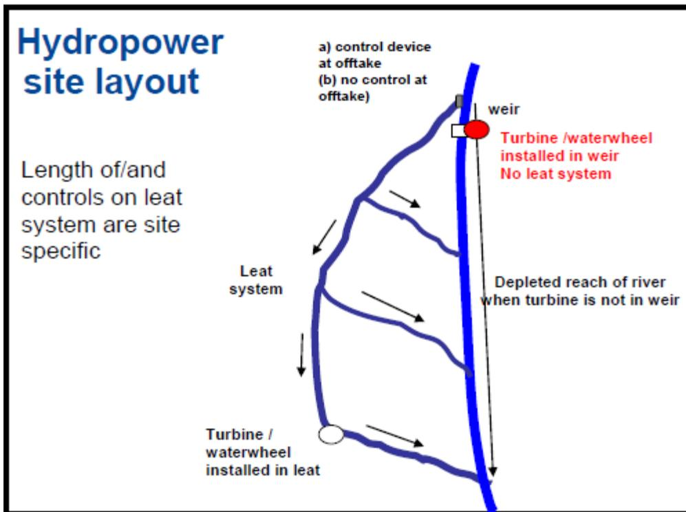
**Figure 4.1 Typical low head hydropower layouts. From Environment Agency (2012)**
