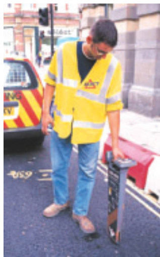
Use of the Cable Avoidance Tool (CAT) to locate underground services (Source: NJUG)
