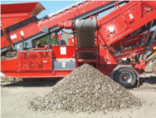
Crushed and graded material from road excavations suitable for re-use as backfill or sub-base in utility trenches
