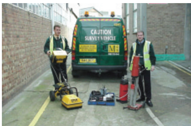
Ground Penetrating Radar (GPR) equipment for the location of underground apparatus (Source: McNicholas Construction Group)
