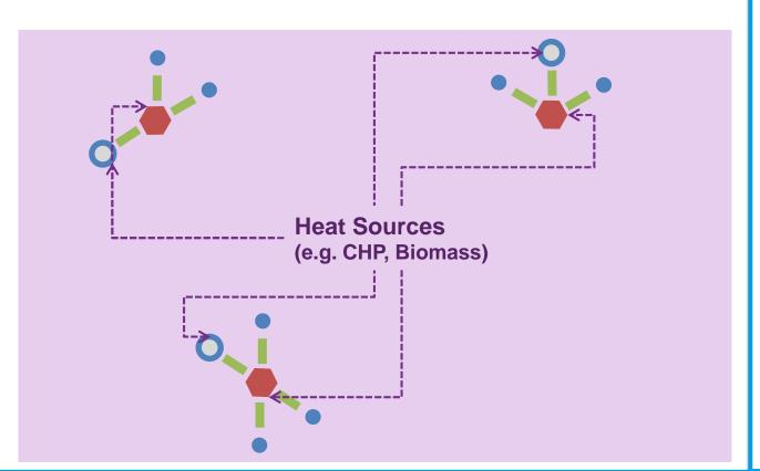
One or more independent cluster networks developed based around key "anchor" loads (e.g. social housing, hospitals, universities etc.) and other loads in the vicinity. Each cluster served by a single, small heat source (e.g. gas CHP, EfW plant, etc)
