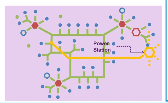
Original heat sources will have reached the end of their lives. These will be replaced with new heat sources, which may include surplus heat from power stations, carried via high capacity transmission mains.
