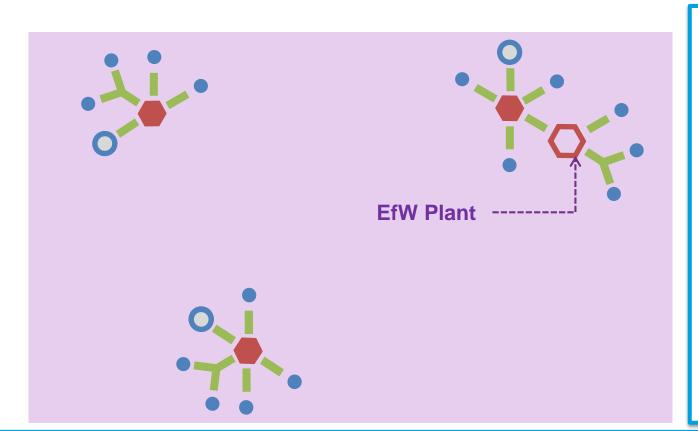
Clusters expand as they become more established to connect additional loads that have become economically viable. Individual heat sources grow in capacity to meet demand or are reinforced with larger heat sources (e.g. EfW CHP)
