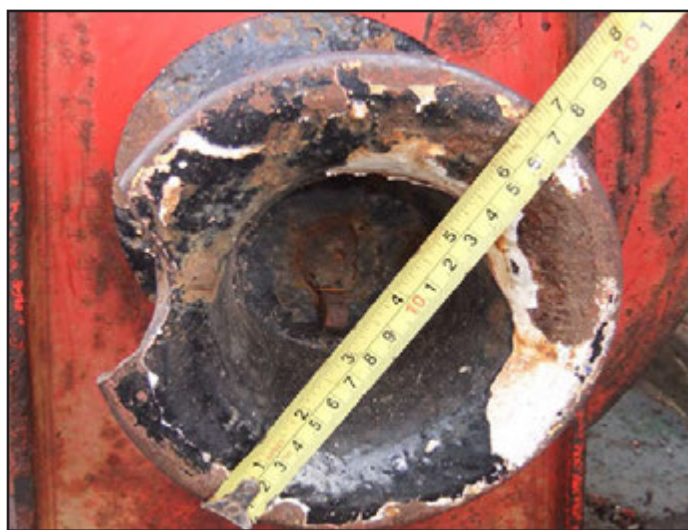
Figure 3: Chunk of cast steel broken from the rim of the starboard warping drum
