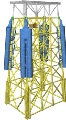
Figure 10. Location of the buoyancy tanks attached to DP2 jacket
