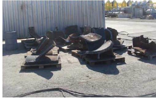
Figure 70. Part of nodes cut out from the DP1, DP1 and QP jackets ready to be sent to the laboratory
