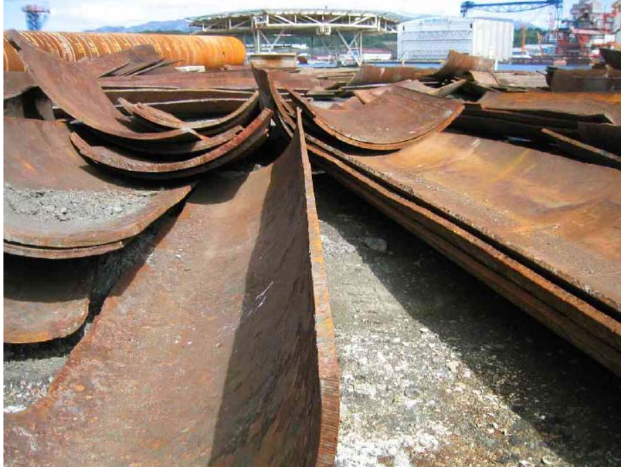
Fig 7.15 Gas-Cut Heavy Walled Tubulars Ready for Recycling
