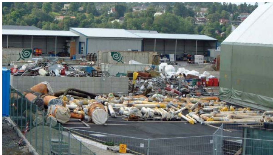
Fig 7.16 Temporary Storage for LSA Contaminated Pipe
