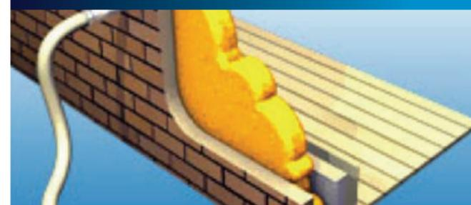
In most houses built after 1930, the external walls are made of two layers with a small air gap or 'cavity' between them; this results in a considerable amount of heat being lost. Cavity wall insulation fills the gap with an insulating material, which reduces the amount of heat that escapes through the walls and helps prevent condensation.
