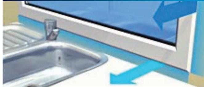
Draught-proofing means blocking up unwanted gaps that let cold air in and warm air out. The most common places where gaps lead outside are: windows; doors; loft hatches; electrical fittings on walls and ceilings; suspended floorboards; pipework leading outside; and ceiling-to-wall joints.
