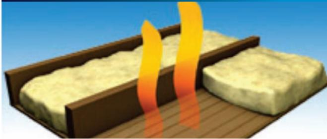
Loft insulation acts as a blanket, trapping heat rising from the house below. For optimum efficiency, pipes can be insulated at the same time. Some properties already have some loft insulation but you could increase this level to the optimal 30cm/12inches to further reduce your energy bills. Your existing loft insulation may also have deteriorated over the years.
