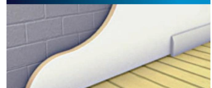
Older properties, usually built before 1930, do not have cavities that can be filled. Internal solid wall insulation reduces the amount of heat that would otherwise pass through your walls and be lost. Plasterboard laminates backed with insulating material (with a total thickness of around 9cm) are fitted directly to the inside of those walls that face the outside. NB: this insulation does not require you to decorate the whole house.
