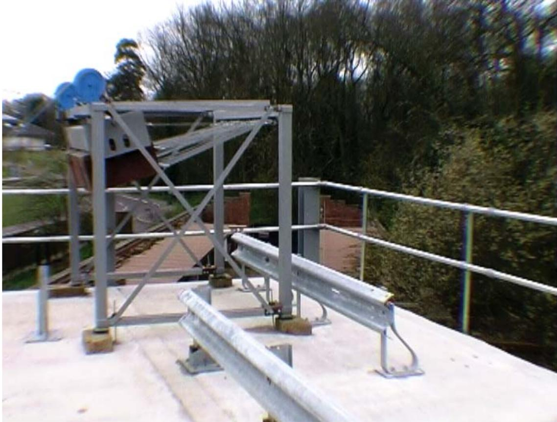
**Figure 1. A suitable dynamic proof test apparatus.**
