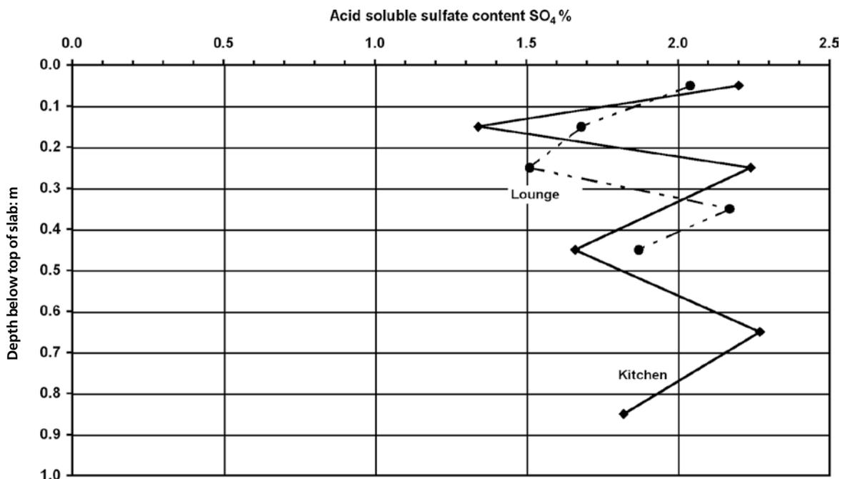
**Figure 2:** Acid-soluble sulfate contents in burnt colliery spoil (red shale) sampled at depths below a concrete floor slab in a 40 year old house. The values, which represent the total amount of sulfates present in the hardcore, vary erratically with depth from 1.3 to 2.25 per cent  $\text{SO}_4$ , reflecting the original variability of the hardcore.
