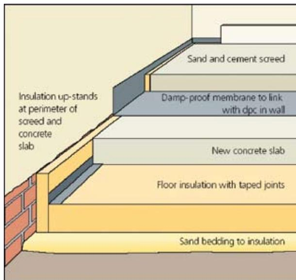
**Figure 10:** Floor slab construction with insulation conforming to Building Regulations Approved Document L1B (from CE 184).
