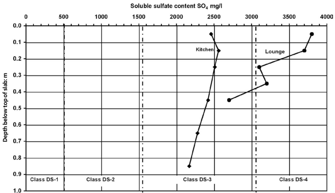
**Figure 3:** Water-soluble sulfate contents in burnt colliery spoil (red shale) sampled at depths below a concrete floor slab in a 40 year old house. Also shown are the Sulfate Class Limits from BRE SD1:2005. The profiles show values of sulfate which increase upwards. This is likely to be due to these soluble sulfates being drawn upwards by water passing through the slab to the warm rooms above.
