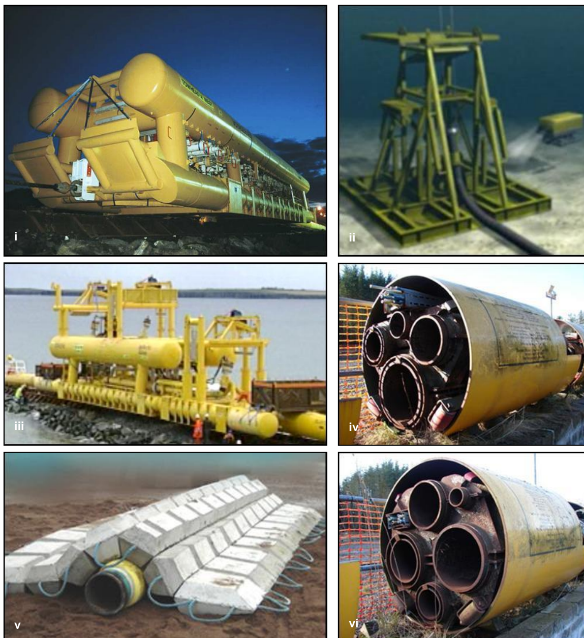
(i). Towhead structure; (ii) Riser base; (iii) MLS; (iv) North Bundle; (v) Mattress; (vi) South Bundle
