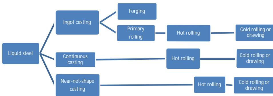
Figure 5: Iron and steel secondary process routes
