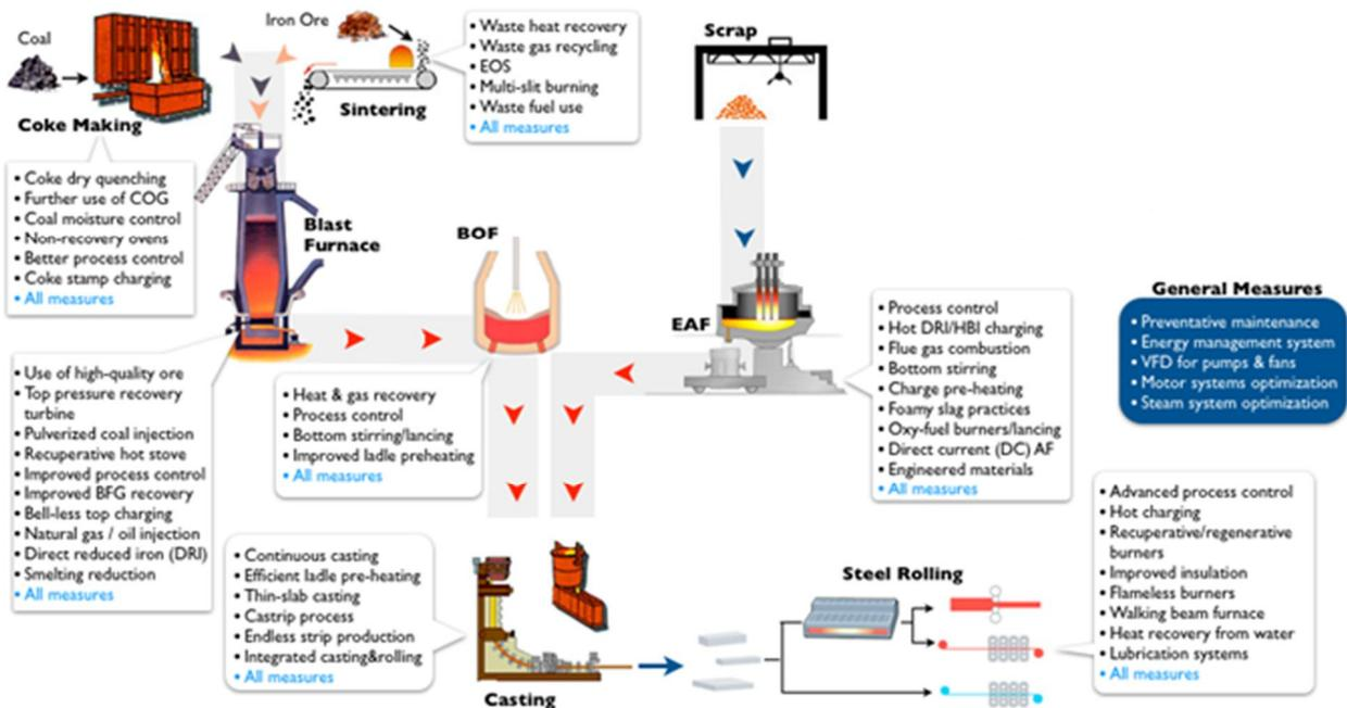
Figure 10: Schematic of iron and steel production processes (IIP, 2014)
