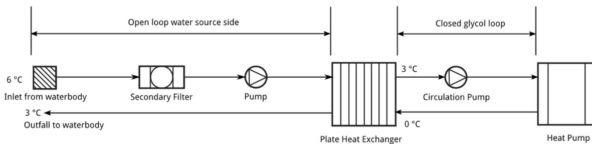
**Figure 23 Schematic of a water source heat pump**
