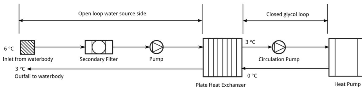
**Figure 23 Schematic of a water source heat pump**
