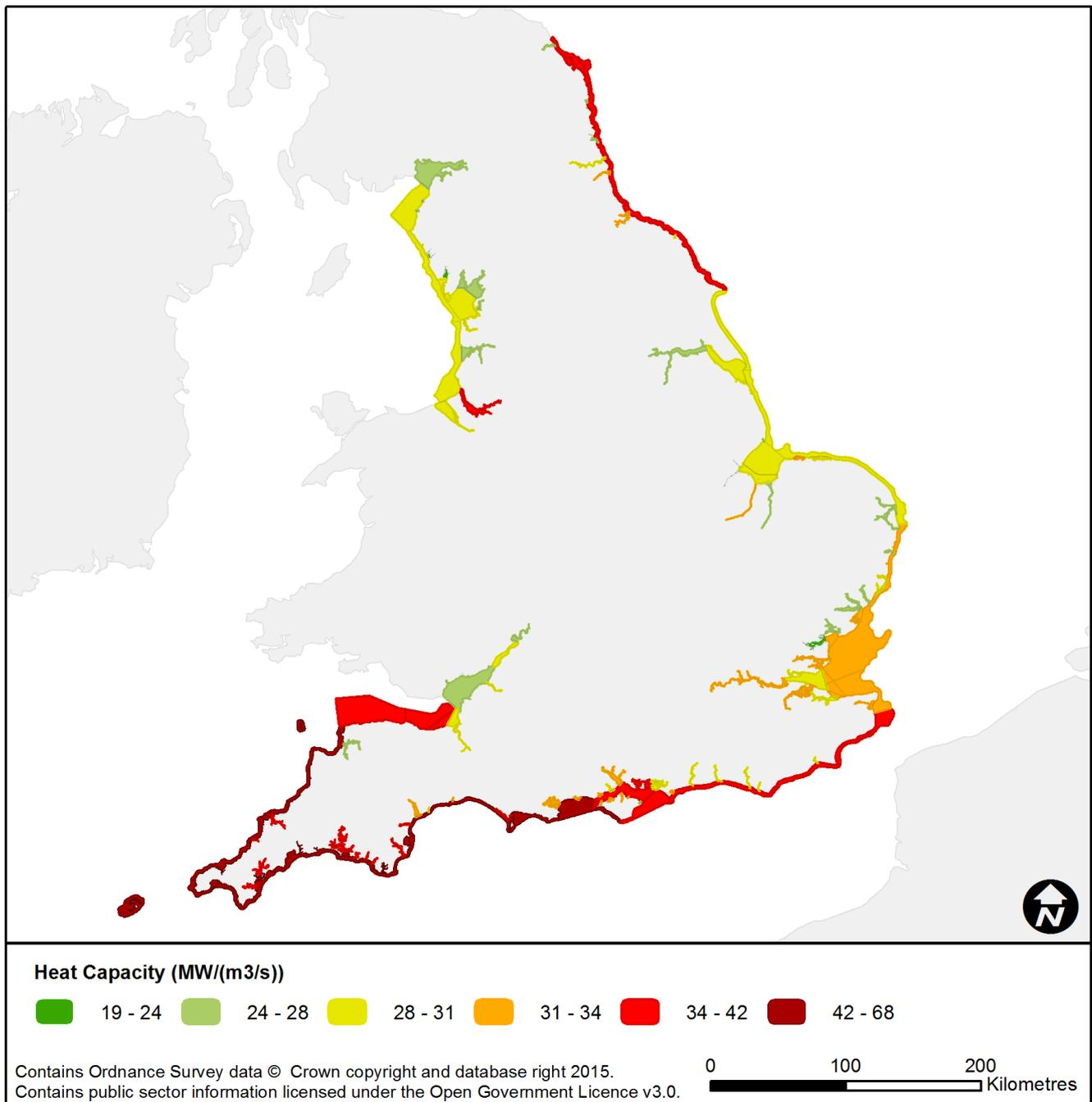
**Figure 19 Heat capacity per unit abstraction for coastal and transitional waterbodies**
