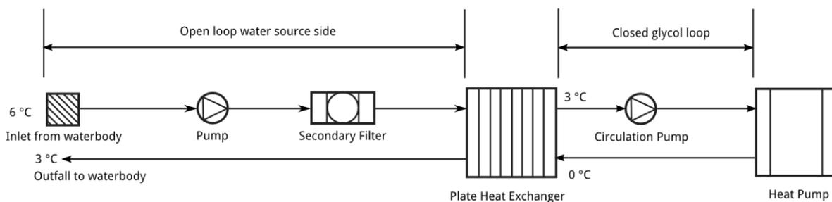
**Figure 9 Heat pump schematic**
