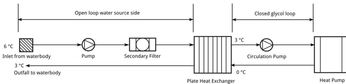
**Figure 9 Heat pump schematic**
