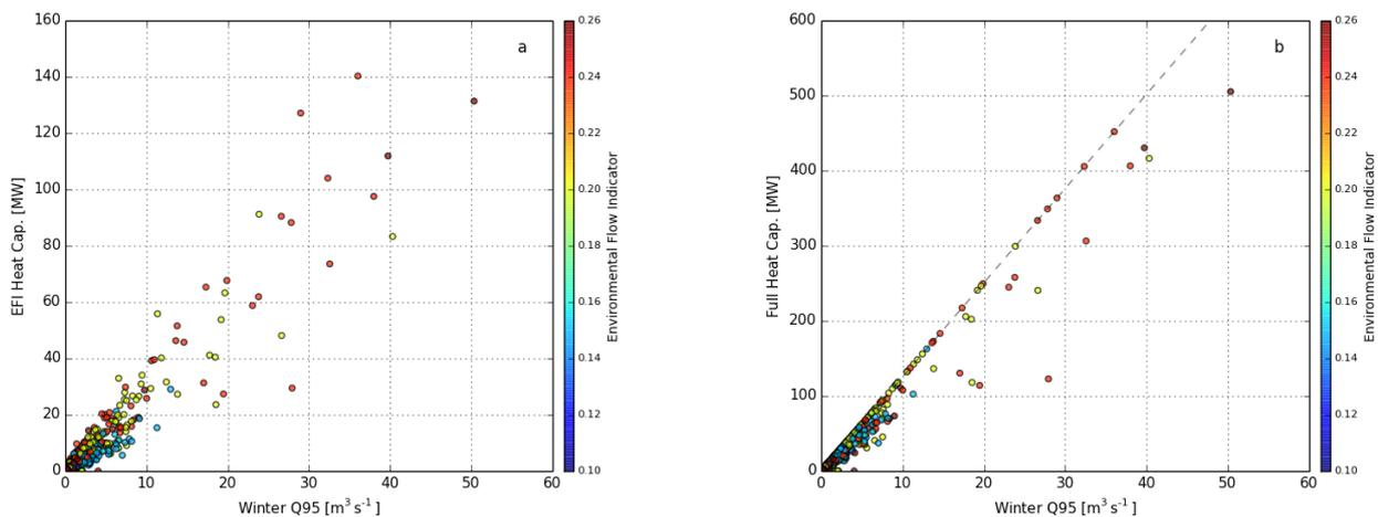
**Figure 12 Relationship between river flow and heat capacity**
