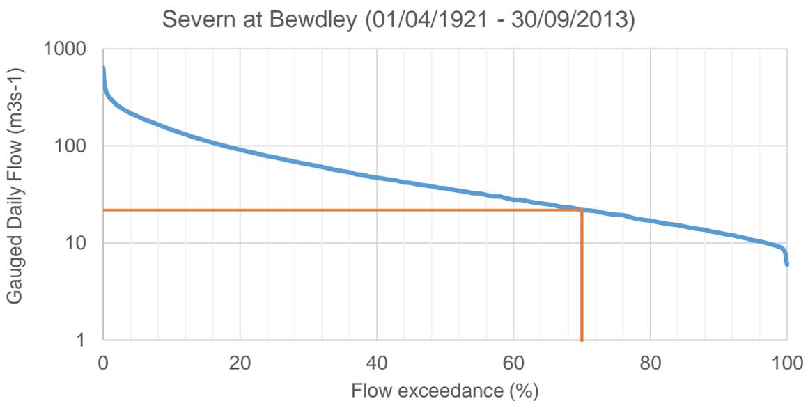
**Figure 1 Example flow duration curve in blue, the orange line explains Q70 as the gauged daily flow equalled or exceeded 70% of the time.**
