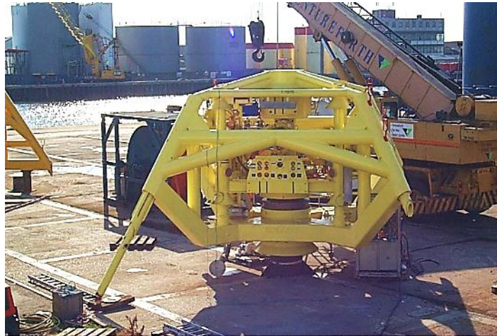
Figure 3.2: Rose wellhead protection structure and Xmas tree
