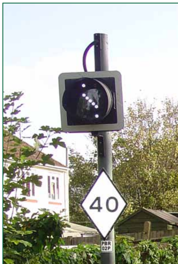
Figure 2 : Points position indicator - points correctly set
