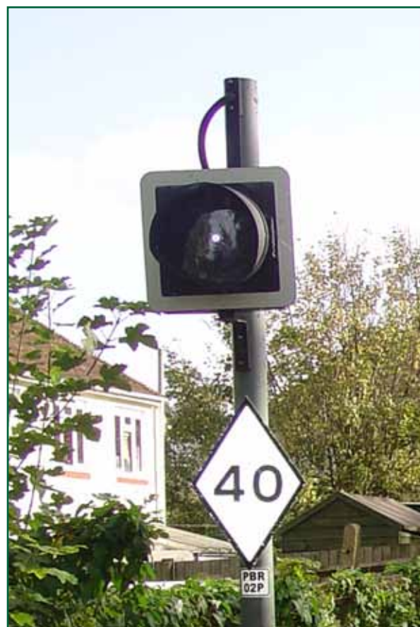
Figure 3: Points position indicator - points not correctly set
