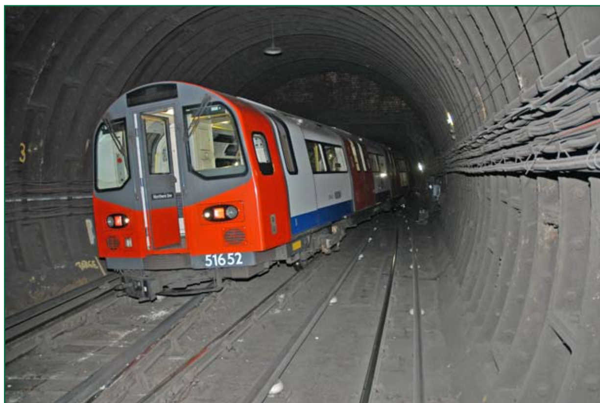
Figure 2: The derailed train seen from the rear.
