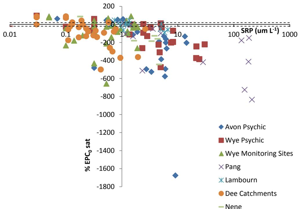
**Figure 2.11** Compilation of  $EPC_{0sat}$  results plotted against SRP concentrations at the time of sampling
