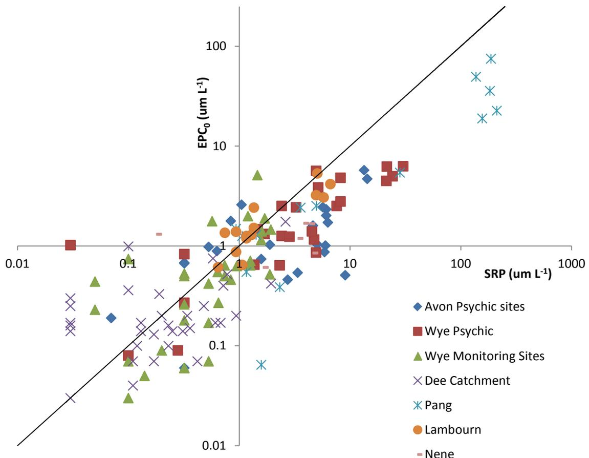
**Figure 2.10** Compilation of  $\text{EPC}_0$  results plotted against SRP concentrations at the time of sampling
