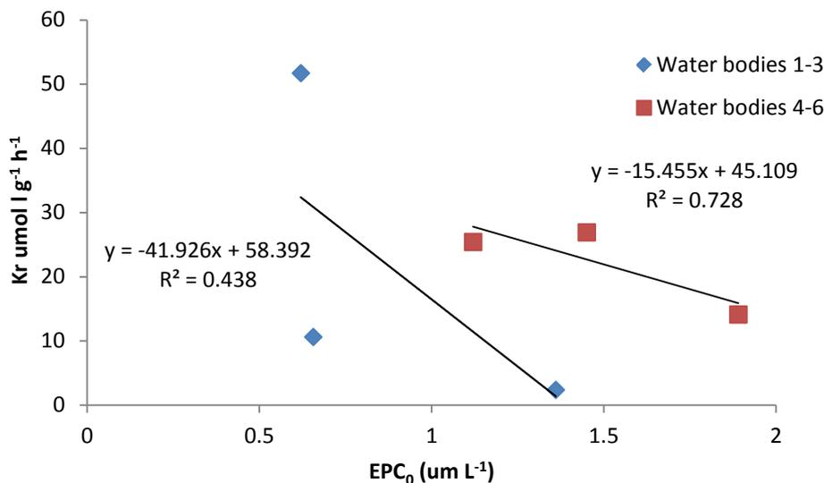
**Figure 2.12 Relationship between rate constant for SRP sorption and  $EPC_0$  for River Nene**
