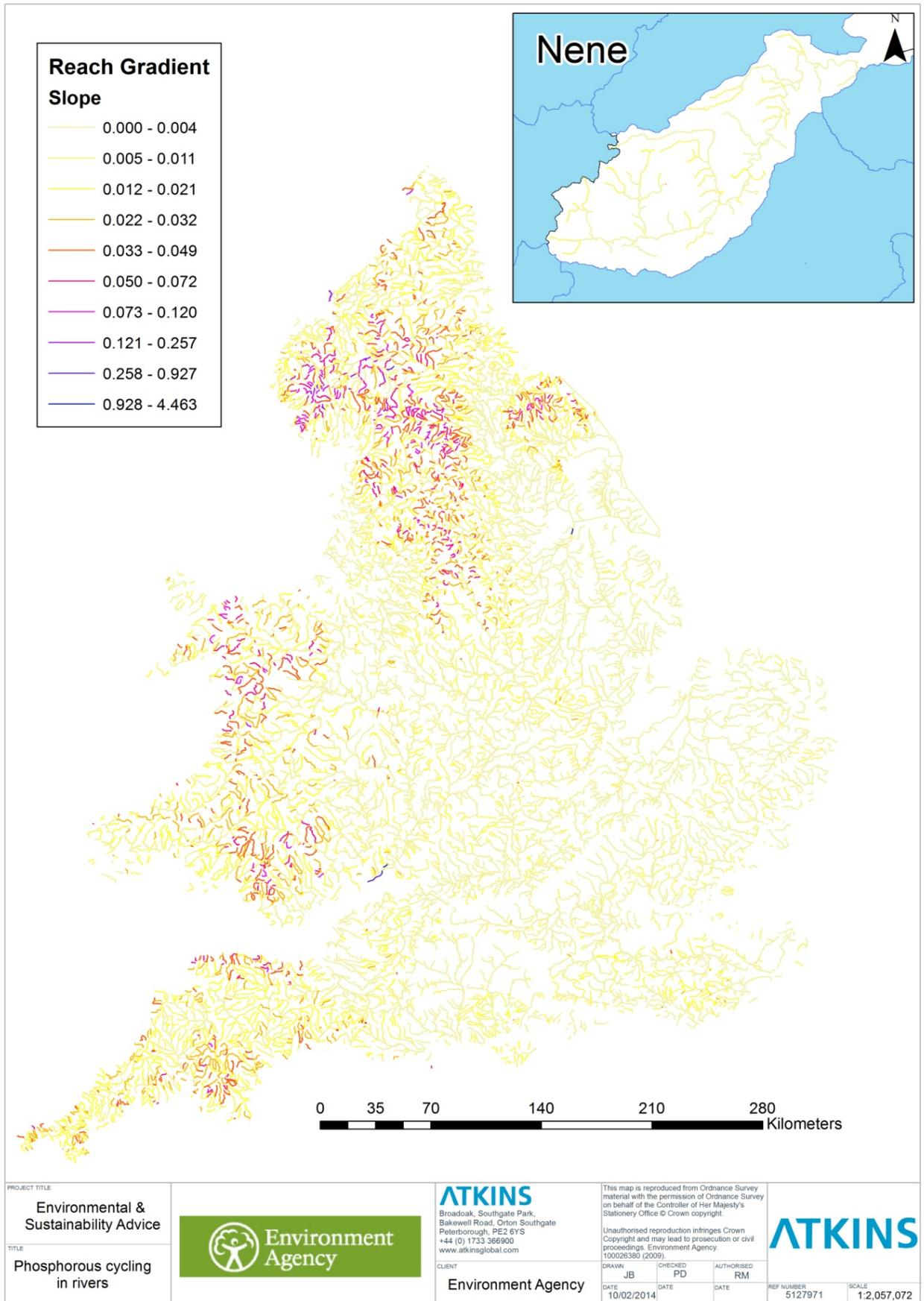
**Figure 4.1 Slope determined for individual river reaches**
