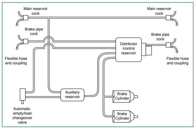
Figure 14: Schematic diagram of the brake system fitted to wagons MAR17712 and MAR17725
