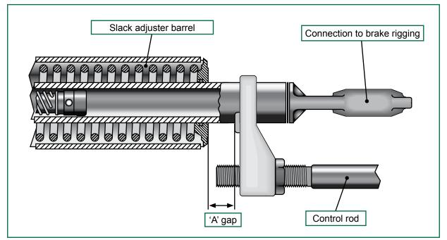
Figure 15: Slack adjuster 'A' gap
