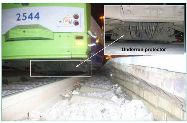
Figure 7: Front of tram showing underrun protector
