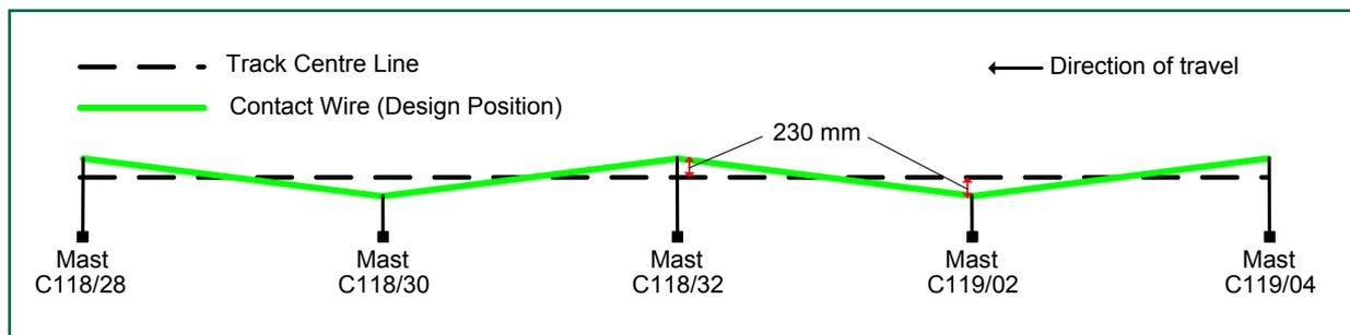
Figure 10: Overhead line designed stagger at accident location
