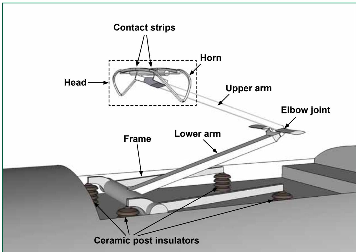
Figure 8: Illustration of train pantograph
