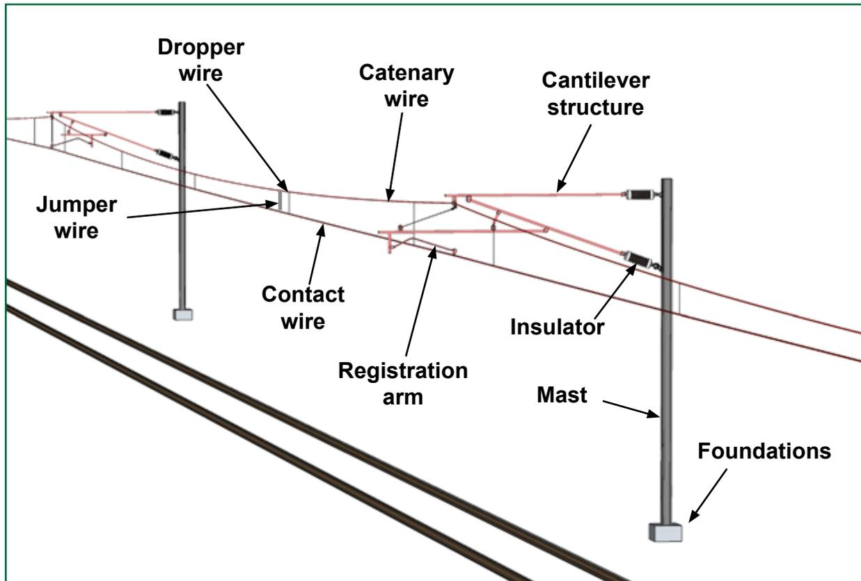
Figure 9: Illustration of overhead line detail
