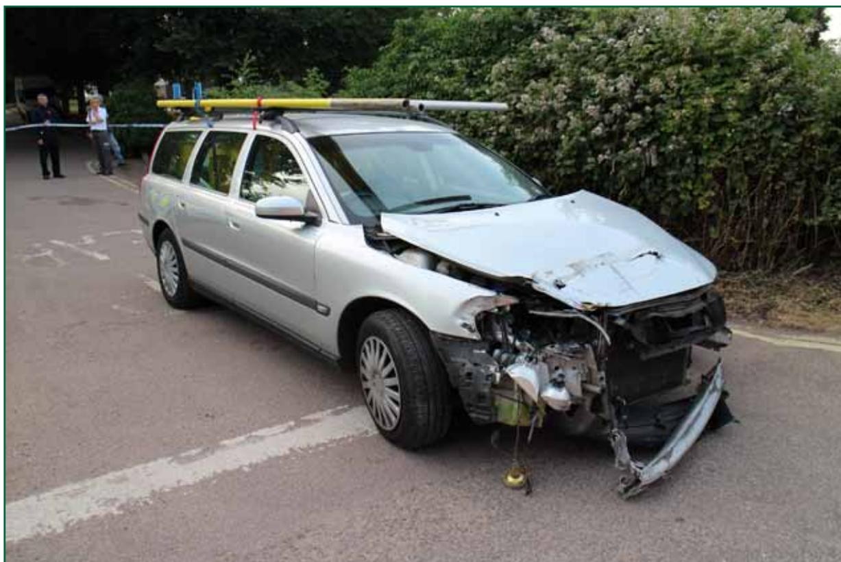
Figure 7: Damage to front of car (photograph courtesy of Network Rail)
