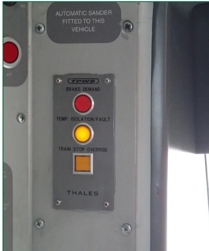
Figure 12: TPWS control panel in unit 165026
