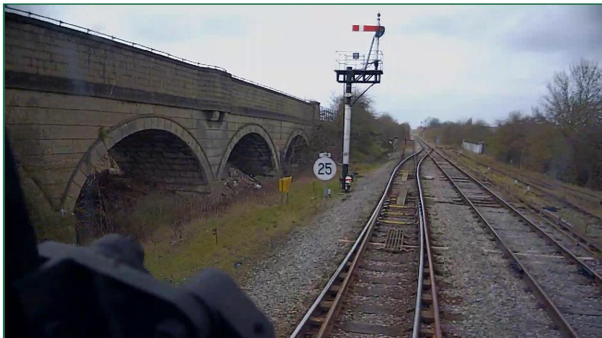
Figure 8: signal GE50 and the start of the single line, showing the trap points.
