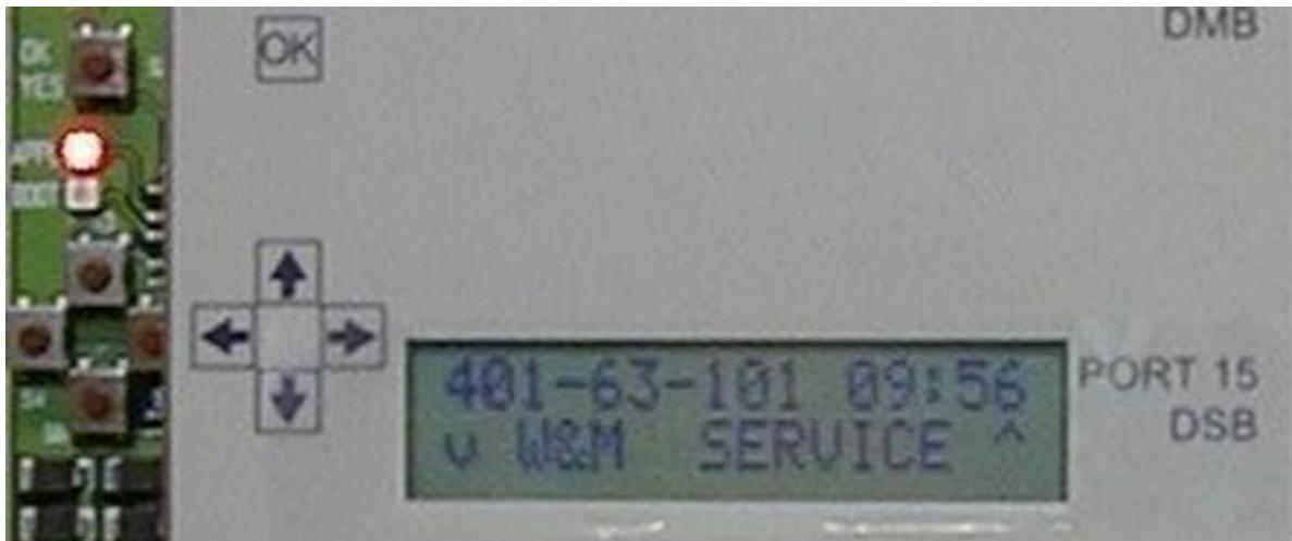
**Figure 16** Central Processing Board (CPB508) display and menu navigation keys
