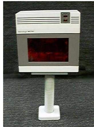
**Figure 10 Typical bar scanners**
