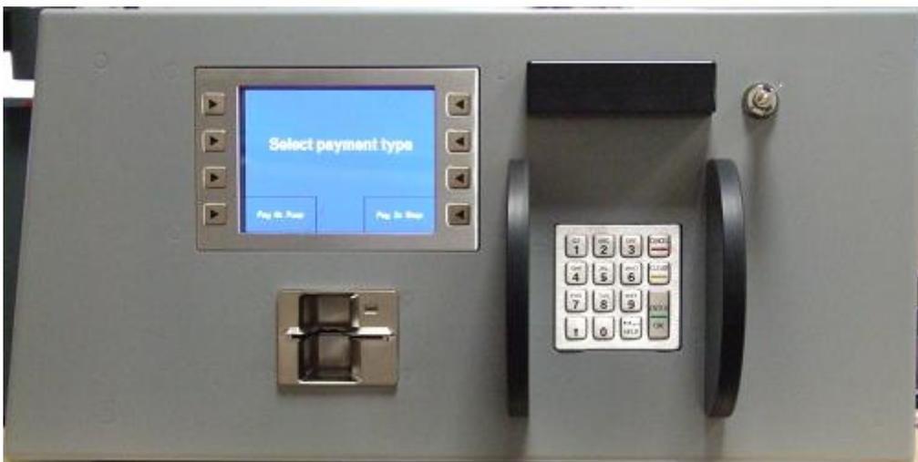
**Figure 19** Wayne CRIND using the Spot M3
