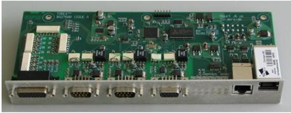
**Figure 23 Control / PSU Board**
