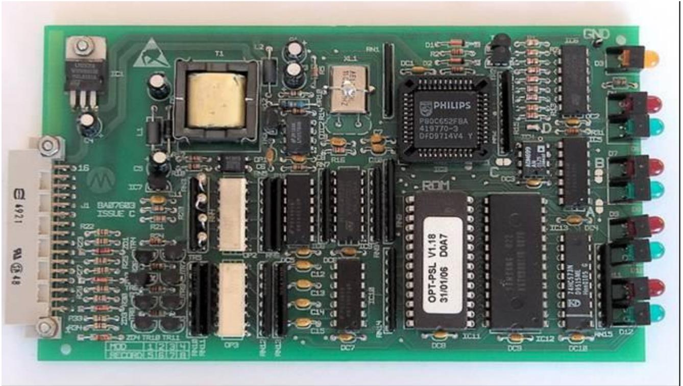
Figure 25 Torex Dispenser Interface Card type BA07603
