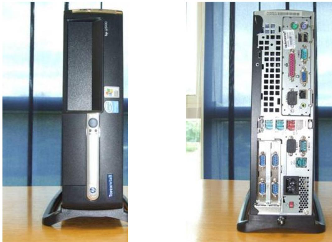
**Figure 14 Hewlett Packard RP 5000 POS PC (front and rear views)**
