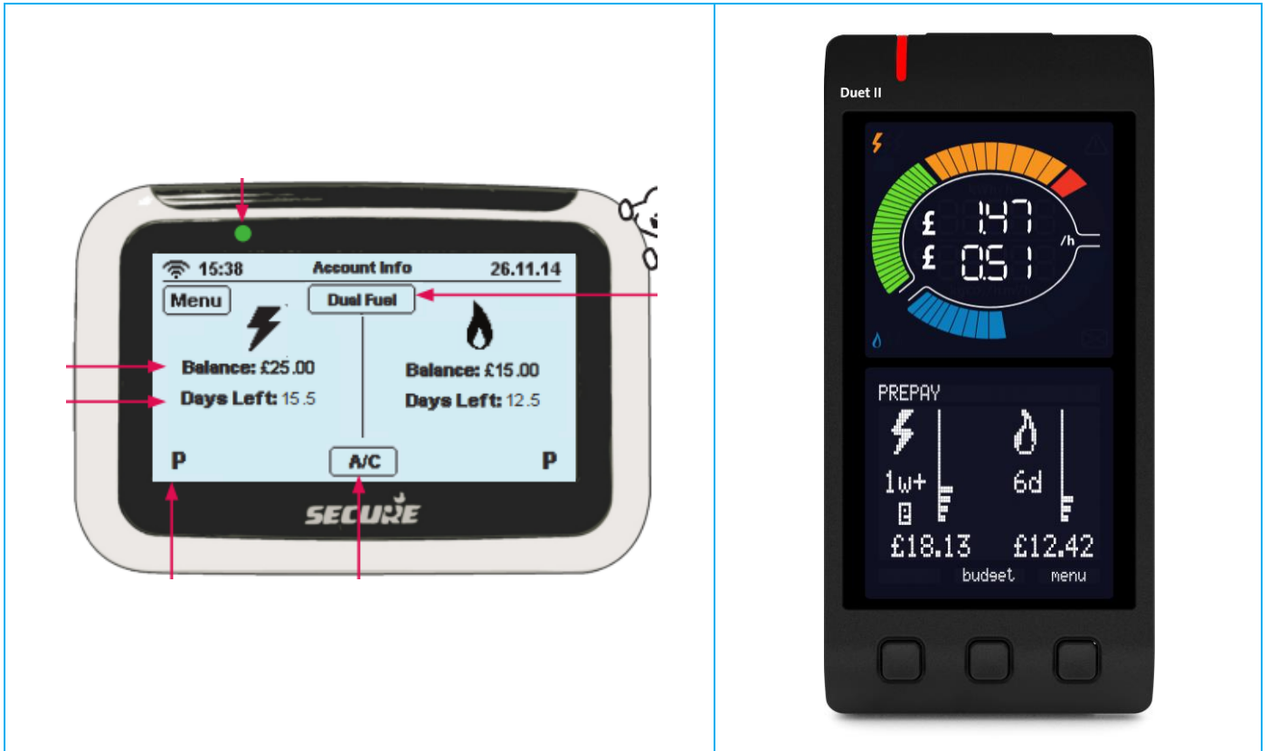
Figure 5: Smart pre-payment IHD default screen and an alternative model's screen that combines the two
