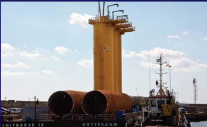
Transition pieces - Lowestoft Port
