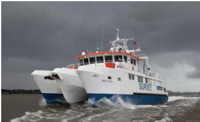
Osiris Projects’ specialist semi-SWATH DP1 survey vessel ‘MV Bibby Tethra’
