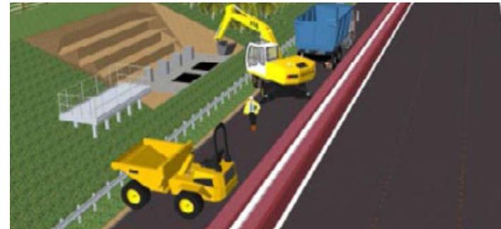
BIM used to plan interface between plant and persons
