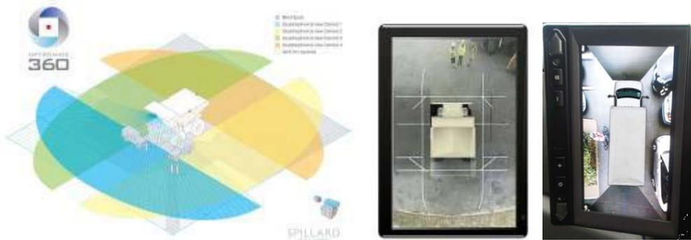
There are even cameras which can determine the human form for other inanimate objects and upon doing so will trigger an alarm in the cab of the plant both on the display unit and also using visual/audible means.
