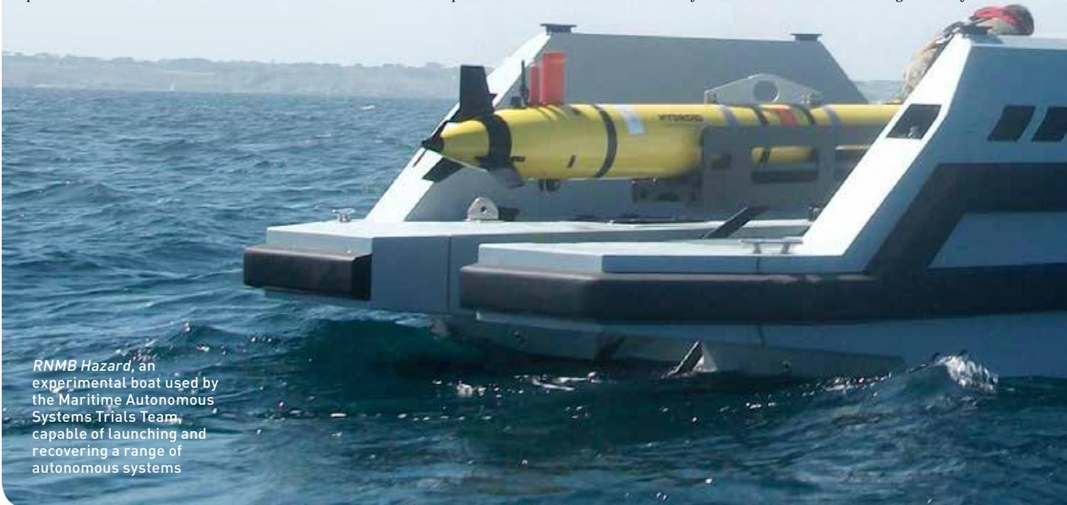
*RNMB Hazard*, an experimental boat used by the Maritime Autonomous Systems Trials Team, capable of launching and recovering a range of autonomous systems
