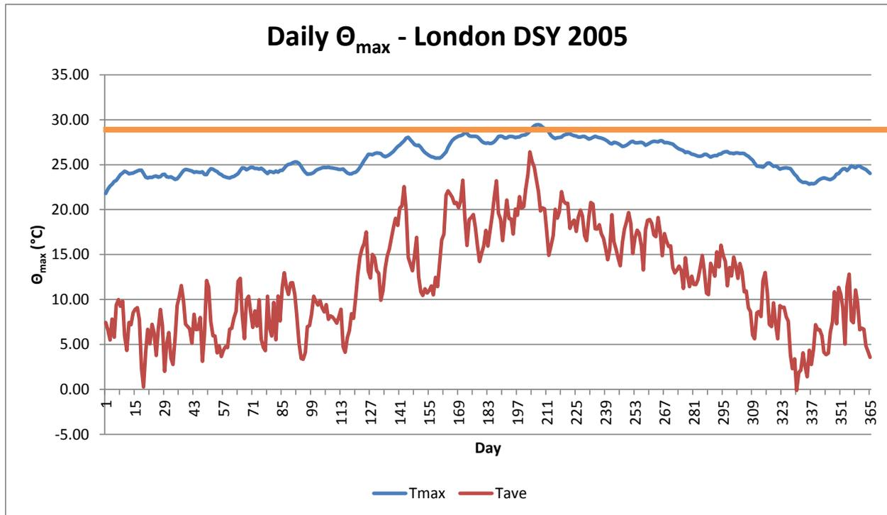
It can be seen from the graph that  $\Theta_{max}$  follows the overall trend of the mean outdoor air temperature, but as it is calculated from the running mean of the air temperature, outlying peaks and troughs are smoothed to form a more uniform temperature target over the course of the year.
