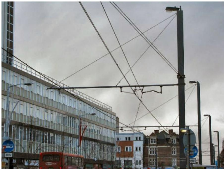
**Figure 1 Tramway OLE Support Structure**
