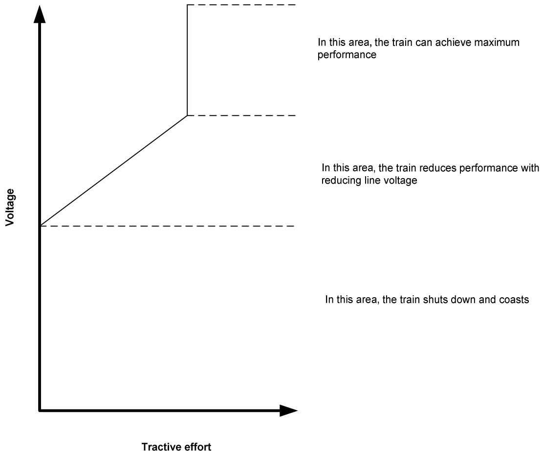
**Figure 6 Tractive effort versus voltage of a typical electric train**
