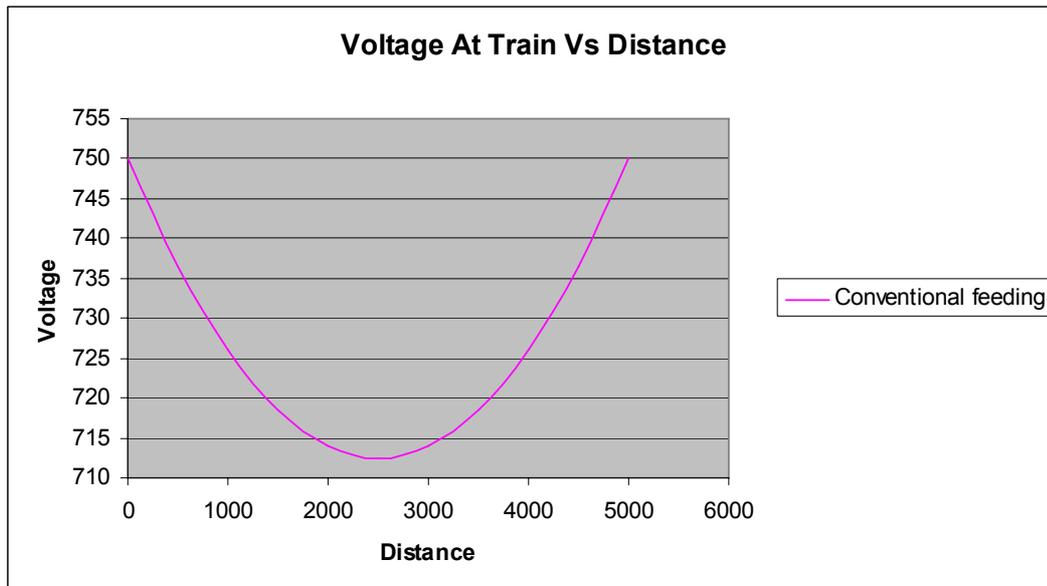
**Figure 8 Voltage versus distance for conventional feeding**
