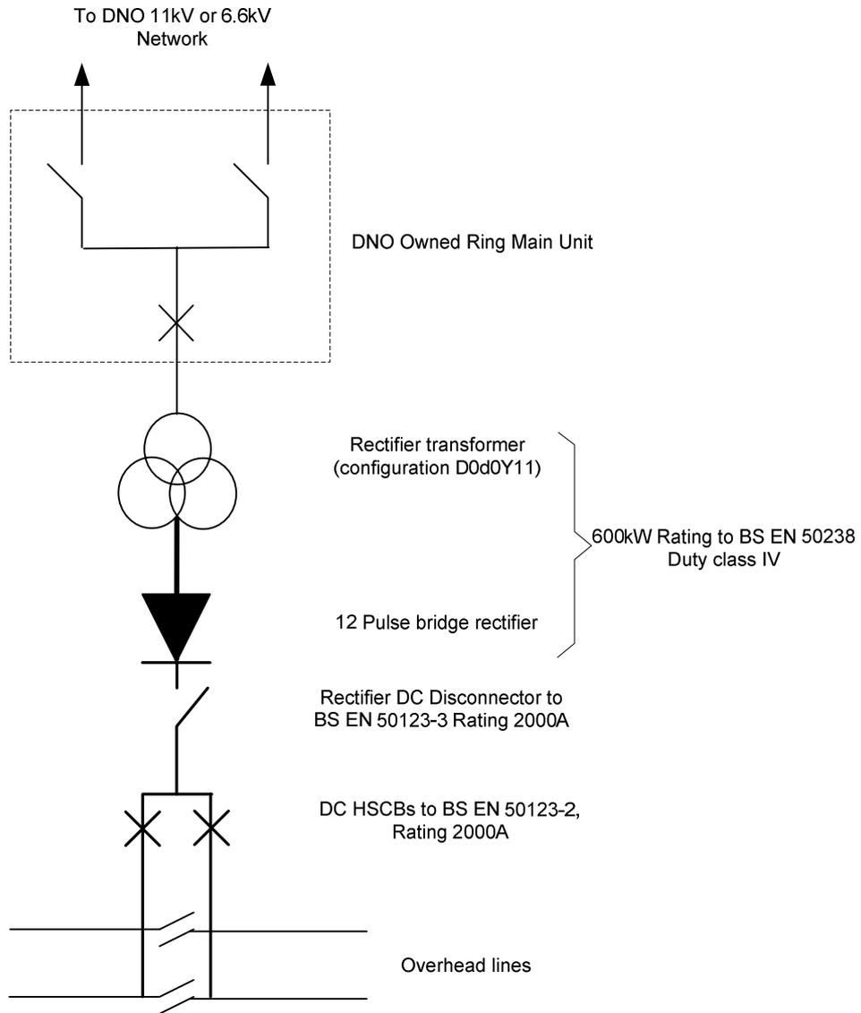
**Figure 14 Proposed Traction Substation Configuration**
