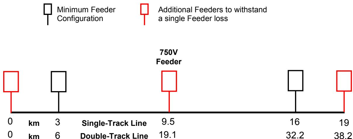
**Figure 4 750V DC Branch Line Feeder Configuration
