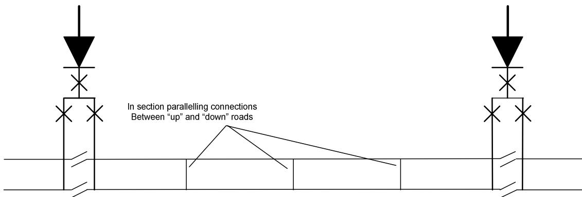
**Figure 12 “Tramway” feeding with in section paralleling**
