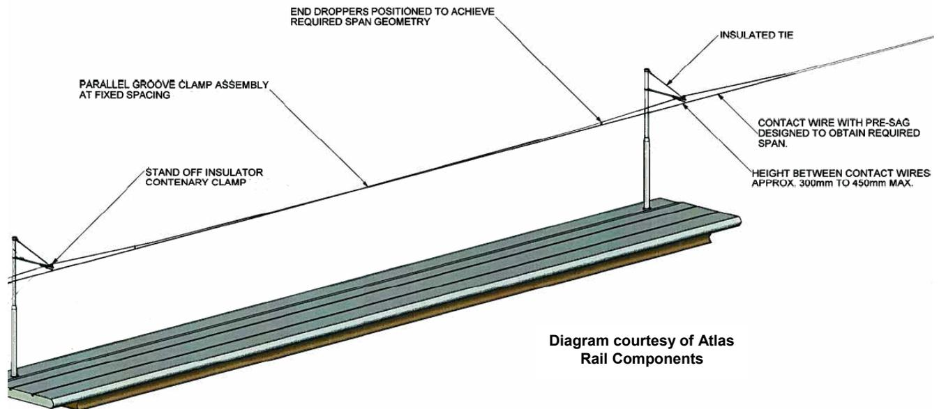
**Figure 2 Hybrid OLE Configuration**
