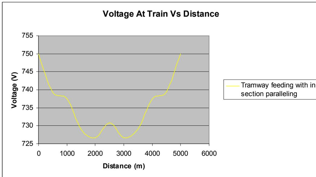
**Figure 13 Line Voltage Profile for Tramway Feeding With In-section Paralleling**
