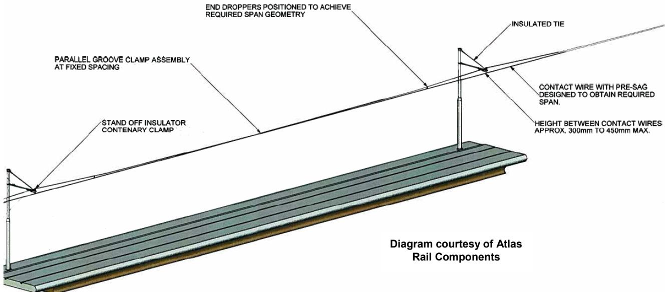
**Figure 2 Hybrid OLE Configuration**
