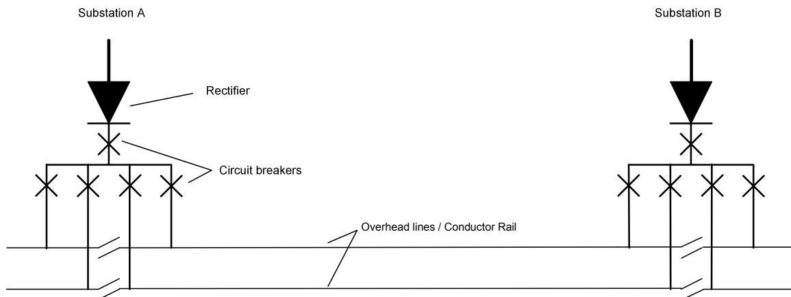
**Figure 7 Diagram of “Conventional” DC Feeding**
