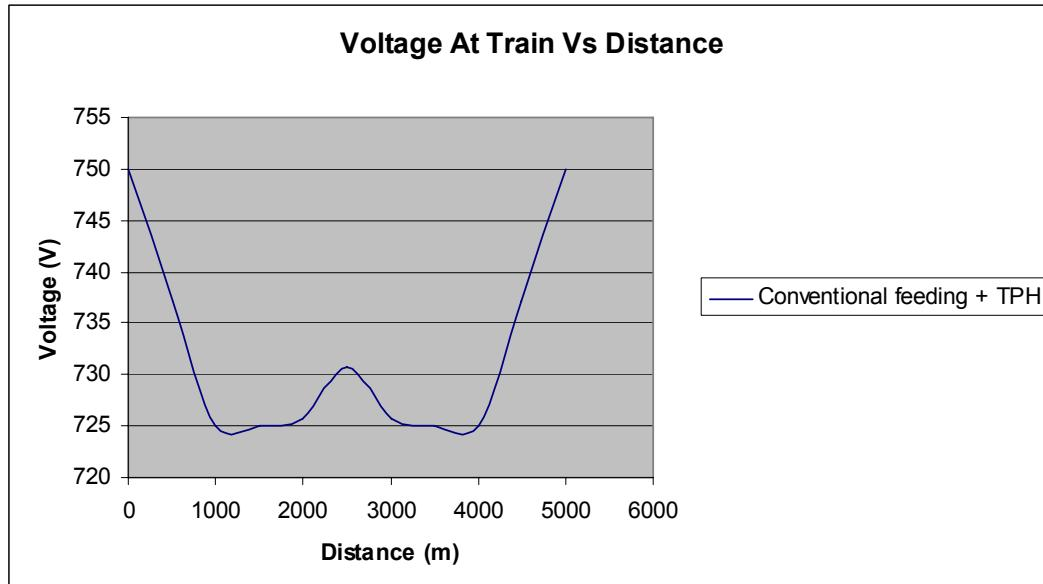
**Figure 10 Voltage versus distance for conventional feeding**
