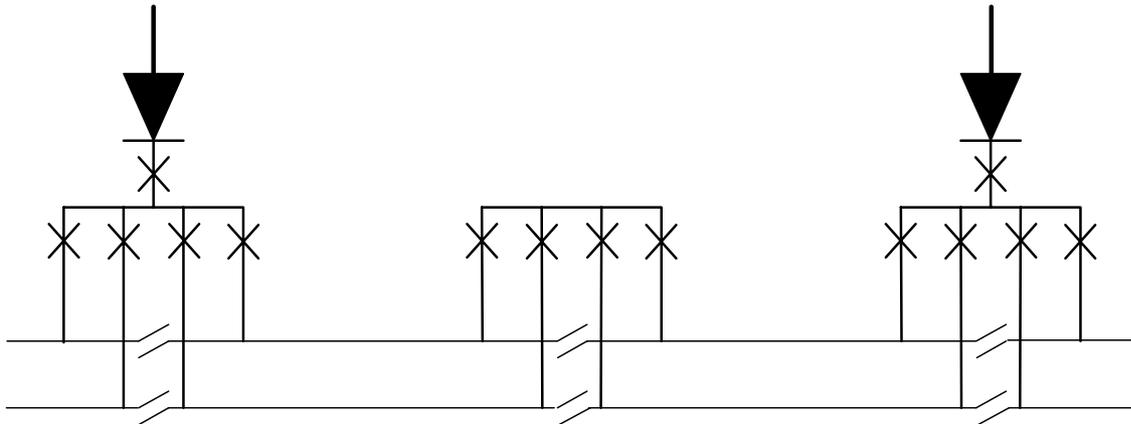
**Figure 9 Conventional feeding with mid point paralleling**
