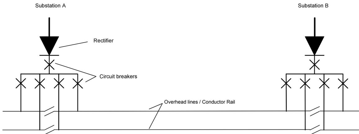
**Figure 7 Diagram of “Conventional” DC Feeding**
