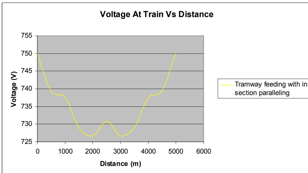
**Figure 13 Line Voltage Profile for Tramway Feeding With In-section Paralleling**
