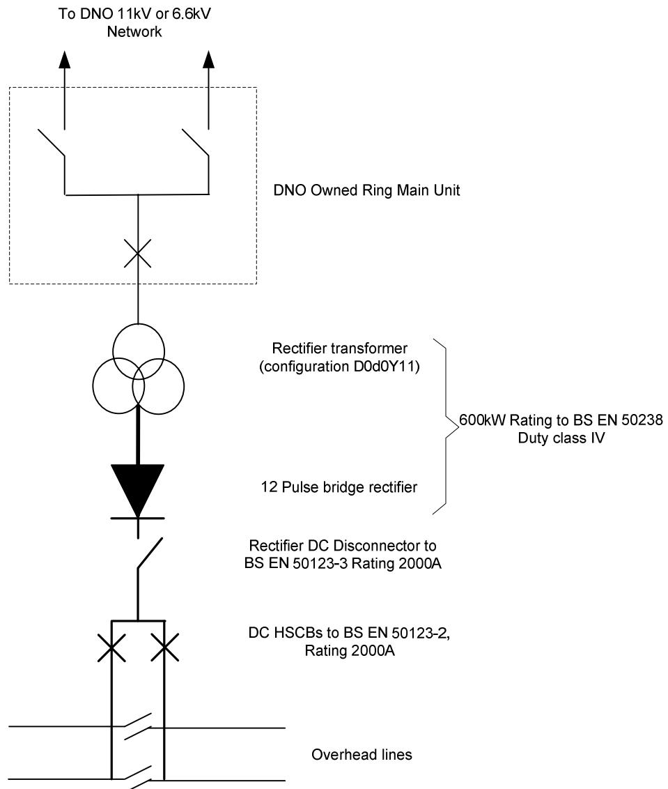
**Figure 14 Proposed Traction Substation Configuration**
