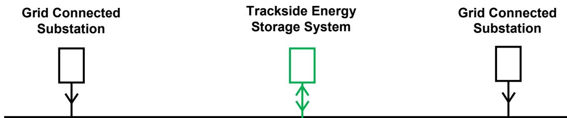
**Figure 5 Branch Line Traction Supply Configuration utilising Trackside Energy Storage**
