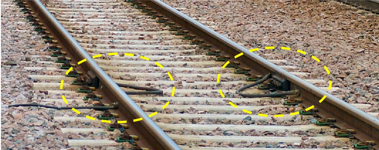
**Figure 15 Jumpers Across Fishplated Rail Joints**
