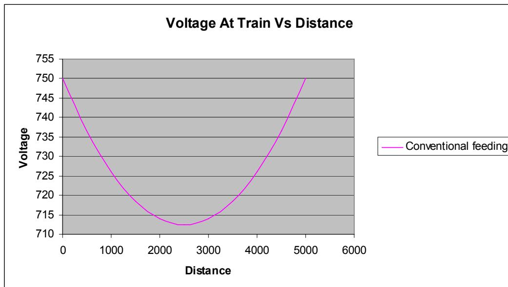
**Figure 8 Voltage versus distance for conventional feeding**
