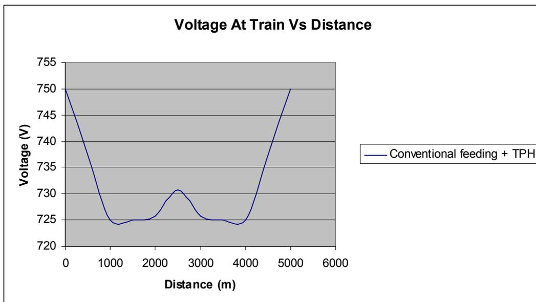
**Figure 10 Voltage versus distance for conventional feeding**
