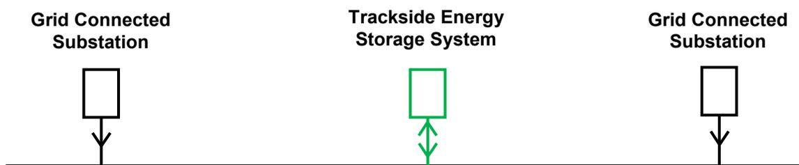
**Figure 5 Branch Line Traction Supply Configuration utilising Trackside Energy Storage**
