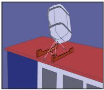
However, had the liferaft floated free, it would not have automatically inflated because its painter had not been attached to the HRU's weak link. The liferaft had also been stowed upside down in its cradle. This would have allowed water to build up inside its canister, reducing its inherent buoyancy and increasing the likelihood of its inflation mechanism suffering from corrosion and failing.
