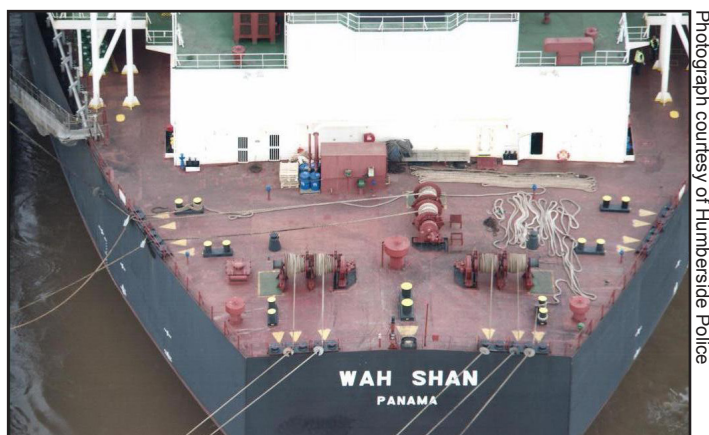
Figure 1: Layout of mooring equipment on the aft deck
