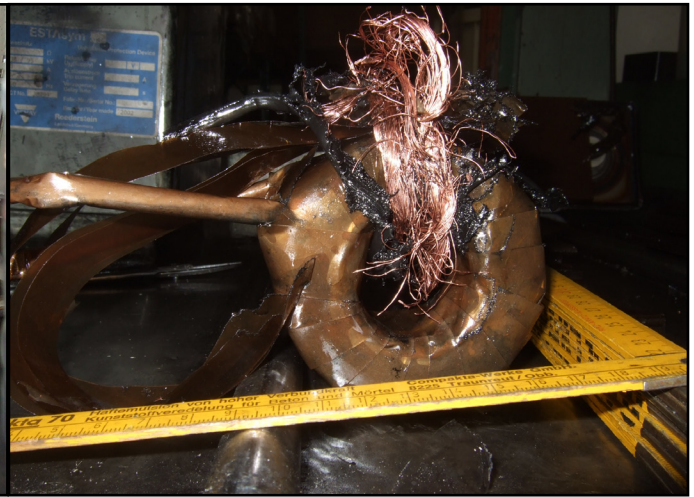
Damaged transformer windings
