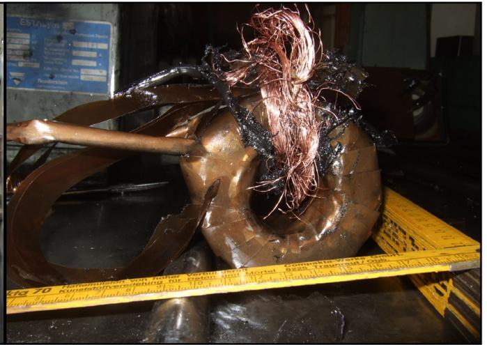
Damaged transformer windings
