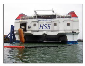
An articulated road tanker crashed through a stern door of the high speed service 1500 (HSS 1500) vessel *Stena Voyager* shortly after the ferry had commenced a scheduled crossing from Stranraer, Scotland to Belfast, Northern Ireland. The vehicle's semi-trailer came to rest on the vessel's port water jet units; its tractor unit remained on the vehicle deck. The ferry was quickly stopped and her crew were able to make the vehicle secure before returning to Stranraer.
