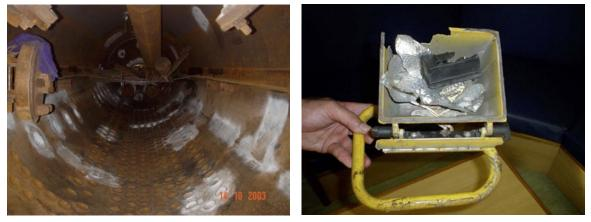
All the evidence points to an accumulation of hydrogen gas in the steam drum which evolved during the cleaning procedure. As the steam drum door was opened, the air combined with the hydrogen to create a mixture that was within the hydrogen explosive limits. As the halogen lamp was introduced, either the hot lens or bulb, or an electrical spark from the lamp ignited the mixture, causing the explosion.
